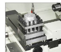
▲ Electrical 4 way toolpost
