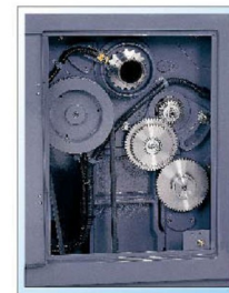
▲ End gear train & Sensor
