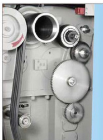
▲ Multiple threading system for cutting worm.
